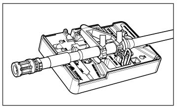
**GAS BLOCK:** Gas blocks come in many sizes and shapes. The standard A2 gas block has three removable pins: two 1/8" pins and one 5/64" pin. The gun barrel and gas block assembly can be placed on the bench block in two orientations for added convenience while removing or installing pins.
