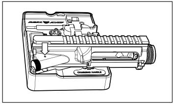
**FORWARD ASSIST:** To remove the pin from the forward assist, position upper receiver as shown. Be sure to depress the forward assist as you align the take down peg into the square hole in the block. Holding the forward assist in this compressed position removes the force on the roll pin. Use a 3/32" punch to remove or install pin.
