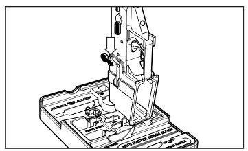
**BOLT CATCH:** The bolt catch has a 3/32" roll pin that can be removed by placing the lower receiver in a vertical orientation. With the pivot pin in the pulled-out position, mount the receiver onto the block. Press the pivot pin in to lock the receiver into the block. Use a 3/32" punch to remove the roll pin.
