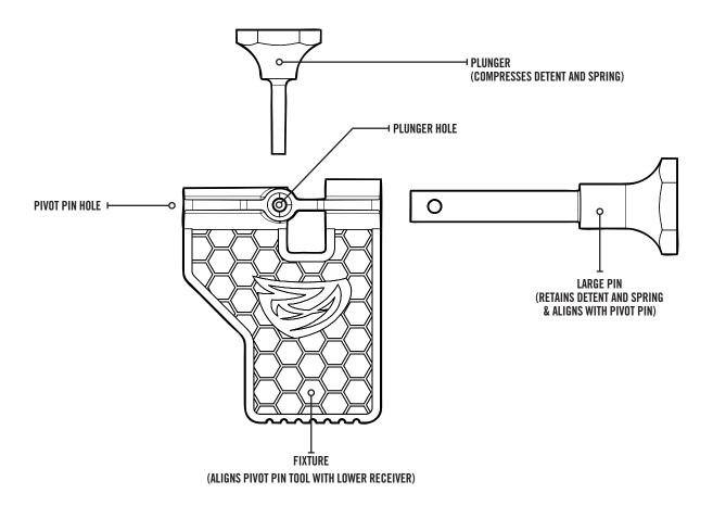
**SAFETY:** Before using the AR15 Pivot Pin Tool on a firearm, you must MAKE SURE THAT THE FIREARM IS UNLOADED AND SAFE to work on. To make installation of the pivot pin easier, we recommend that you place your lower receiver in a properly secured magwell vise block. It is your responsibility to exercise caution during the use of this tool.
