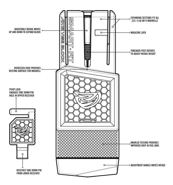
**SAFETY:** Before using the Smart-Fit AR15 Vise Block on a firearm, you must MAKE SURE THAT THE FIREARM IS UNLOADED AND SAFE to work on. To avoid damaging your firearm, make sure that you are using a properly secured bench vise to hold the Smart-Fit Vise Block in place during use. It is your responsibility to exercise caution during the use of this tool, especially when applying torque.
