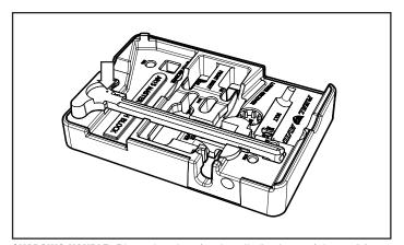
**CHARGING HANDLE:** Place the charging handle in the upright position as shown. Standard charging handles have one 5/64" pin. Custom charging handles can have multiple pins in various locations. Consult charging handle manufacturer for exact pin sizes to reduce the risk of causing damage to the charging handle.
