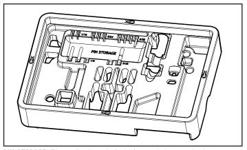
**PIN STORAGE:** Place pins into their designated slots on the bottom side of the bench block for storage during assembly or disassembly. There are also four powerful magnets embedded in the side walls to help capture loose pins as they are punched out.
