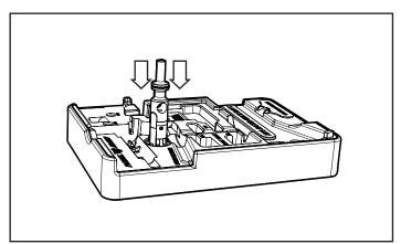
**BOLT GAS RING INSTALLATION:** Place the bolt in the vertical position to install the three gas rings.
