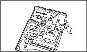
**BOLT EJECTOR:** The bolt ejector is retained by a 1/16" roll pin. The roll pin is under tension from the spring loaded ejector. To relieve the tension, lay the bolt onto the bench block as shown and tighten the bolt ejector compression screw, then remove or install the roll pin. **Note that the precise orientation of the bolt is critical for this process.**
