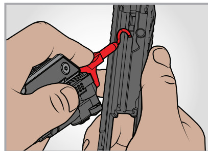
Clean out carbon and gunk from inside action
