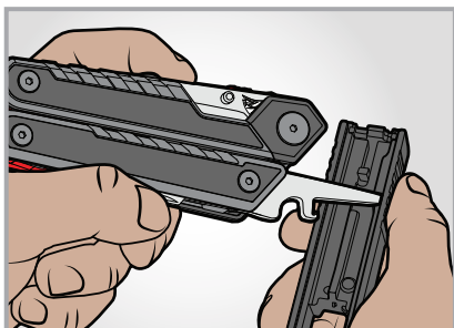
Scrape carbon from bolts
